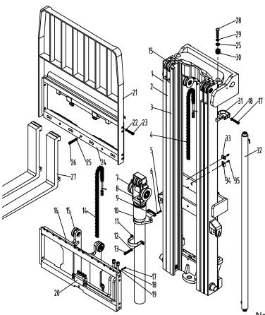
Index 6.00 Note: Y - Separate Illustration No. PART NUMBER DESCRIPTION Qty Remarks Note 24 AC15 15 side-shifter assembly 1 25 Washer16 GB/T93 3 GB/T70.1 26 Screw M16%x25 1 27 CPD20SR-16.3A.6-00 Fork assembly 2 GB/T5785 Screw M16%x1.5%x65 2 29 GB/T95 Washer16 2 30 15803002202 Screw 2 CPD20SR-16.3A-01 Platen 2 31 CPD20SR-16.3A.8-00 Side oil cylinder 2 33 CPD20SR-16.3A-05 Platen 4 4 34 CPD20SR-16.3A-02 Platen 2 1 35 Screw M6%x30 GB/T70.1 6
